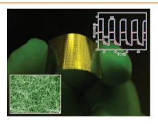
Single-crystalline p-type Zn<sub>3</sub>As<sub>2</sub> nanowires are successfully synthesized and used as building blocks for high-performance field-effect transistors and photodetectors. By using a contact printing process, highly aligned nanowire arrays are produced to fabricate thin-film transistors and photodetectors on both rigid and flexible substrates.
