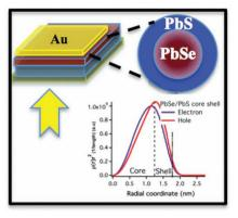
PbSe core and PbSe/PbS core/shell quantum dots (QDs) are employed in a QD/TiO2 heterojunction solar cell. Theoretical calculations show that the wave functions of the electrons and holes are extended to both materials, which contributes to the better photovoltaic performance of the PbSe/PbS core/shell compared to the PbSe core. The PbSe/ PbS core/shell heterojunction solar cell produces a power conversion efficiency of 3.93%.
