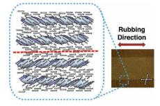
Successful alignment control of the B4 helical nanofilament assembly in a binary mixture system of bent-shaped and rod-shaped liquid crystals is presented. The aligned nanofilament domains appear as extremely smooth and uniform stripes over millimeters. Second-harmonic generation (SHG) studies including a new technique, interferometric SHG microscopy, reveal that in these aligned domains, polarity from the nucleus and chirality are preserved.
