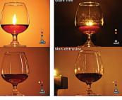
A sensationally warm but physically cold candle-light-style emission driven by electricity is developed in lieu of hydrocarbon-burning in the energy-inefficient, greenhouse gas releasing candles invented 5000 years ago. The dimmable and single-sided emitting nature of the developed candle-light-style organic light-emitting diode (OLED) provides a lighting atmosphere free from glare and obtrusion.
