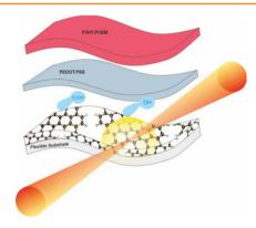
A methodology for controlled in situ reduction of spin-cast graphene oxide nanometric films on flexible substrates and the subsequent realization of highly conductive and transparent electrodes for flexible organic photovoltaic devices is presented. The technique is compatible with temperature-sensitive substrates in the sense that it achieves reduction of films on flexible substrates in a single step.
