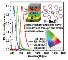
Two coordination complexes with deep blue emission, small singlet-triplet splitting, and ambipolar transport properties are designed and synthesized. Efficient electroluminescent devices with the three primary colors are achieved by employing the complexes as an undoped deep-blue emitter in organic light-emitting devices (OLEDs) and as a host in red and green phosphorescent OLEDs.
